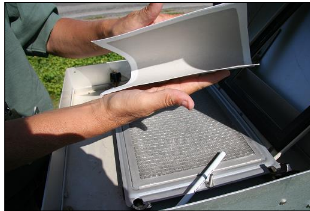
Collecting an exposed filter from a hi-volume particulate monitor
