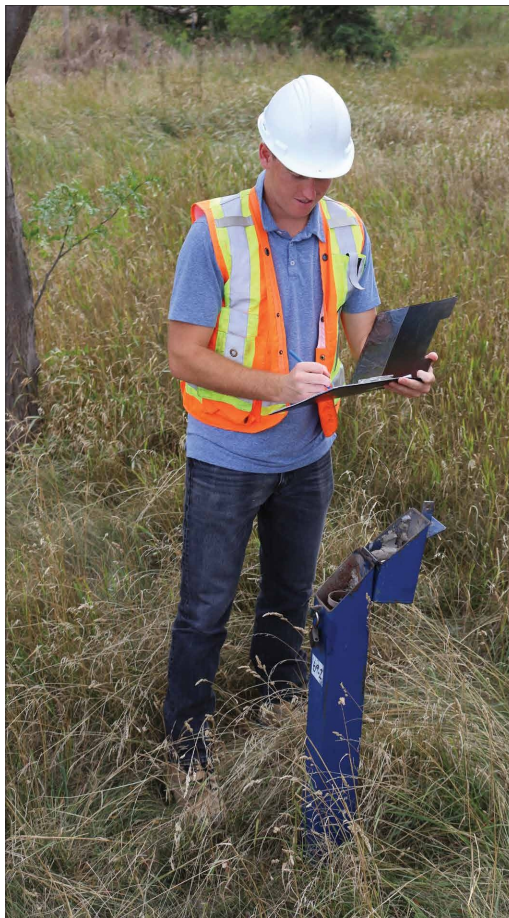
Groundwater monitoring well
