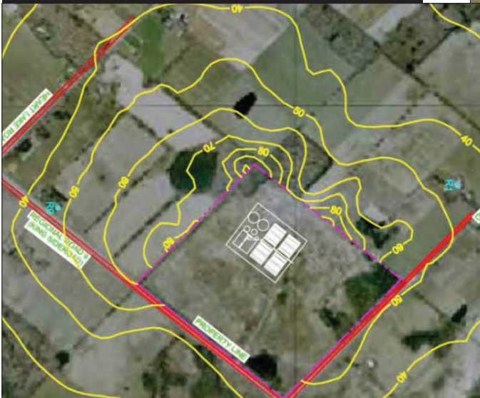
Sample Model of Noise Levels Around a Facility
